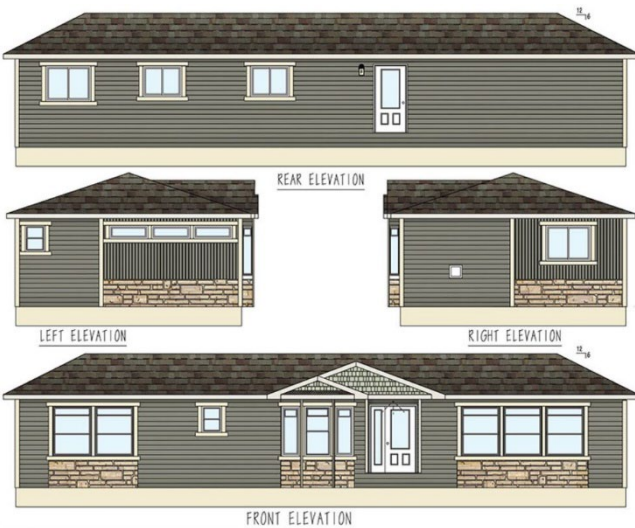
Example of Exterior Elevation
