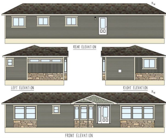
Example of Exterior Elevation
